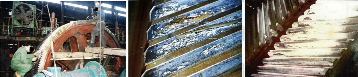
Repair with special Catalina welds + SKODA brand SKODA brand double helical mill reducer sprocket with 128 fully damaged teeth. Some teeth were devastated to the abrasive-terminated bottom diameter.
