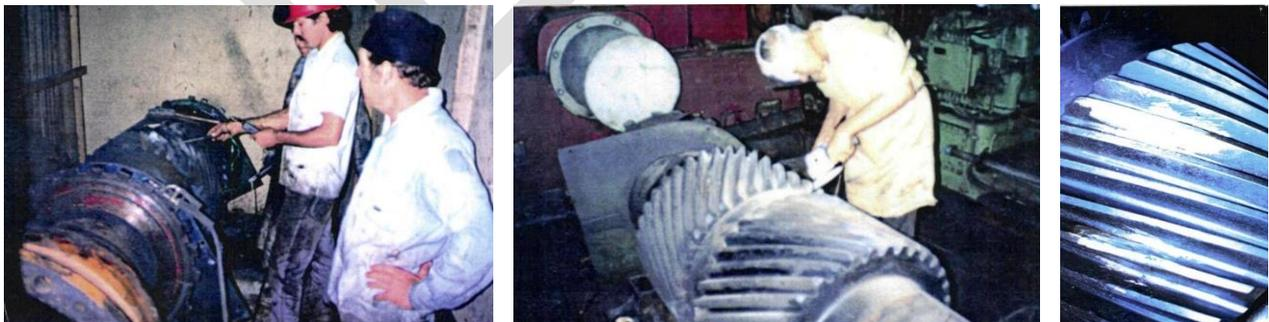
Repair with special welding of sKODA-branded mill reducer pinion with manual abrasive finish.
